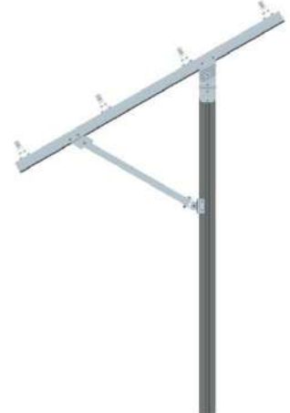
Step 4: Mounting the T-Rails
